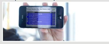
With Journeo's M-EPI solution, real time information can be deployed to stops via QR codes and NFC tags, allowing any user with a smartphone to access an audio departure board, announcing services that depart from a stop.
